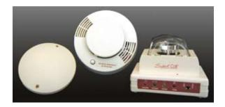
Silent Call is the smoke alarm we provide to people with hearing impairments. It has three separate components: a smoke alarm with a transmitter (model 1008-3), a vibrating disc (model VIB-PJ), and a receiver with or without a strobe light (model SK09214). The alarm provides an audible alert and transmits a signal to the receiver and the strobe light. The receiver then activates the vibrating disc that is under the mattress.
